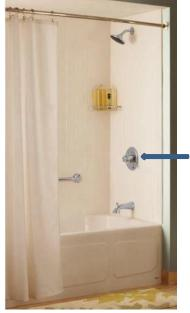
The mixing valve is seen located between the shower head and bathtub faucet spout.
